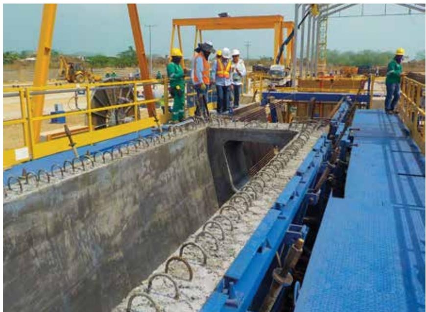
A vibration and heating system ensures steady compaction and curing of the concrete used. V girders in three different lengths, weighing up to 85 t, are currently being produced for the "viaducto Gran Manglar", the longest road bridge in Colombia.
